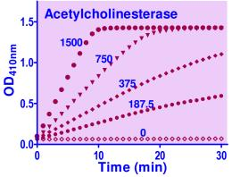
Kinetics of 0-1500 U/L Acetylcholinesterase Reaction in 96-well plate
