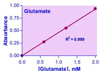
Standard Curve in water measured with PICOEXPLORER™
